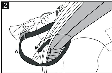
**2 Pass the two ends of the belt (A) around the license plate holder following the direction indicated in the figure.**
