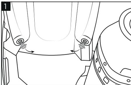
**1 Remove the original screws holding the license plate.**
