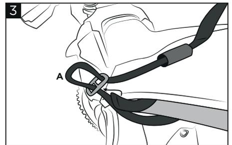
**3 Pass the end of the belt (A) through slot of both buckles, right and left. Follow the instruction in the figure.**
